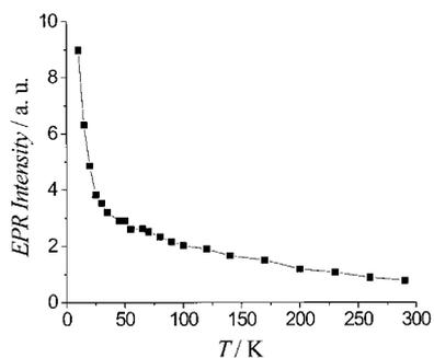
Figure 2. Temperature dependence of the intensity of EPR signal for a powdered sample of **14**.
