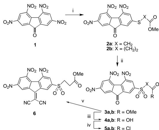
Scheme 1. i) HS-X-CO<sub>2</sub>Me + NaHCO<sub>3</sub>/MeCN, 20 °C, 2–6 h; ii) H<sub>2</sub>O<sub>2</sub>/AcOH, 60–70 °C, 3 h; iii) CF<sub>3</sub>CO<sub>2</sub>H/H<sub>2</sub>O, reflux, 4–6 h; iv) (COCl)<sub>2</sub>/CH<sub>2</sub>Cl<sub>2</sub>, 20 °C, 20–40 h; v) CH<sub>2</sub>(CN)<sub>2</sub>/DMF, 20 °C, 6 h.
