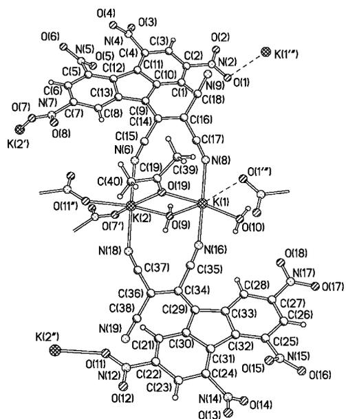
Figure 10. Crystal structure of  $K[23] \cdot H_2O \cdot \frac{1}{2}Me_2CO$  (**23a**). Bond lengths [Å]: K(1)–N(8) 2.398(4), K(1)–N(16) 2.409(4), K(1)–O(9) 2.446(3), K(1)–O(10) 2.262(3), K(1)–O(19) 2.405(3), K(1)–O(1'') 2.728(3), K(2)–N(6) 2.497(4), K(2)–N(18) 2.481(4), K(2)–O(9) 2.391(3), K(2)–O(19) 2.335(3), K(2)–O(7') 2.429(3), K(2)–O(11'') 2.423(3). The disorder of the nitro groups at C(24) and C(25) is not shown.
