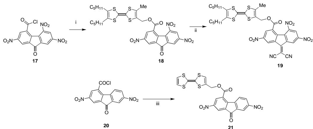
Scheme 4. i) **10** + BuLi, THF, -100 °C → 20 °C, 1 h, then + **17**, -100 °C → -15 °C, 3 h, then -15 °C, 12 h; ii) CH<sub>2</sub>(CN)<sub>2</sub>/DMF, 20 °C, 8 h; iii) TTFCH<sub>2</sub>OH + pyridine/MeCN, 20 °C, 12 h.
