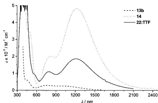
Figure 5. Electronic spectra of compounds **13b**, **14** (in  $\text{CH}_2\text{Cl}_2$ ) and CTC **22:TTF** (in PhCN).
