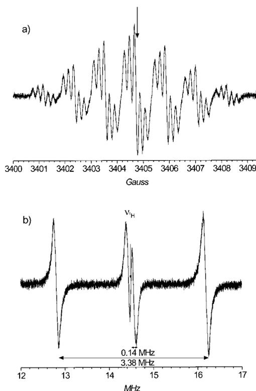
Figure 3. X-band EPR spectrum (a) and ENDOR spectrum (static field corresponding to the middle of the EPR multiplet) (b) of **24** in MeCN/toluene (3:2 *v/v*) solution at 285 K.
