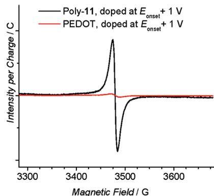
**Figure 3.** X-band EPR spectra of electrochemically doped poly-**11** (solid line) and PEDOT (dashed line) films on Pt wire. The intensities are normalized by the doping charge.
