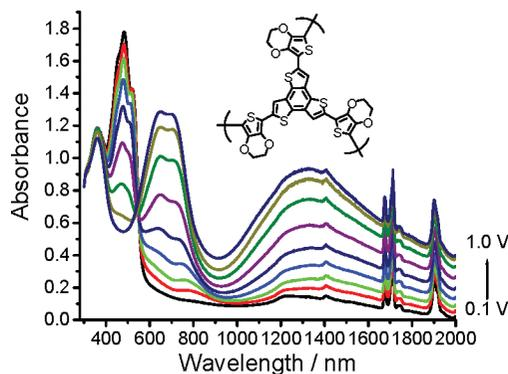
Terthienobenzene (TTB, **6**) was prepared through a new, high yield route along with  $\pi$ -extended derivatives **10** and **11**. Electropolymerization of tris-EDOT derivative **11** results in a highly stable cross-linked conjugated polymer that shows polaron confinement between the TTB units as confirmed by UV–vis–NIR spectroelectrochemistry and EPR.
