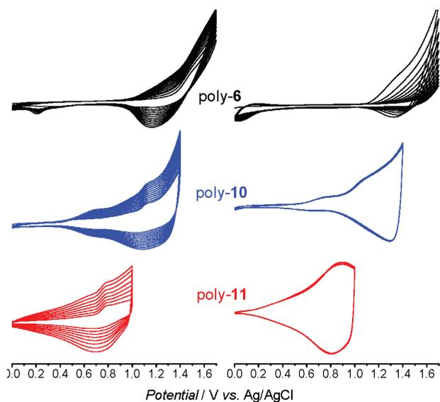
**Figure 2.** (left column) Electropolymerization of **6** (0.02 M in DCM), **10** (0.01 M in DCM), and **11** (7 mM in DCM); (right column) CVs of the corresponding polymer films in propylene carbonate.
